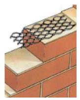
Embedded in the normal thickness of brickwork joint, brickforce gives brickwork increased resistance to tensional stresses - important for buildings erected on reclaimed ground or on other ground in which settlement may occur. Equally suitable as a reinforcement for concrete block work partition slabs, asphalt guttering and in other work.
